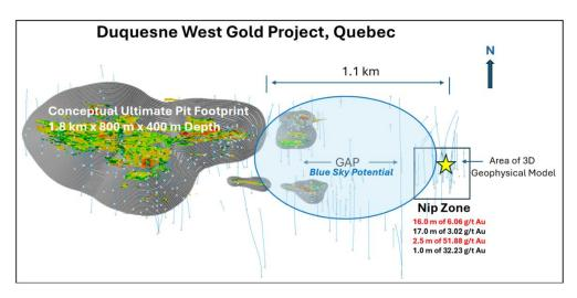
You can see the new target zone (Nip Zone) at the right; on the left is the openpit model. The Nip zone was discovered in 2013 by geophysical tests, but market conditions back then didn't allow for further investigation.
